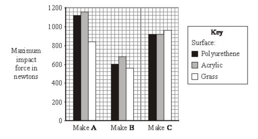
(i) Which **one** of the three makes of running shoe, **A**, **B** or **C**, has the best cushioning system?
