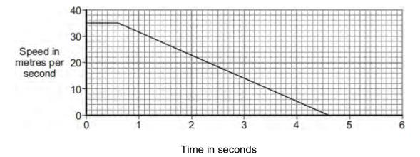
(i) Determine the braking distance.
